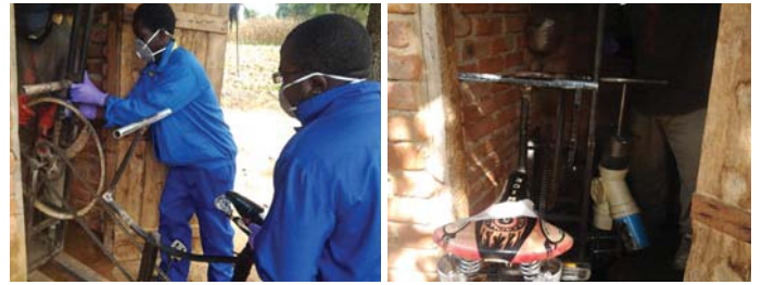
Figure 5: Modified pedal transmission mechanism being carried inside the pit latrine (a) and attached with the Gulper technology inserted in the sanitation keyhole (b).
